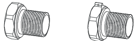
(1) Connector without hole for sealing (2) Connector with hole for sealing
