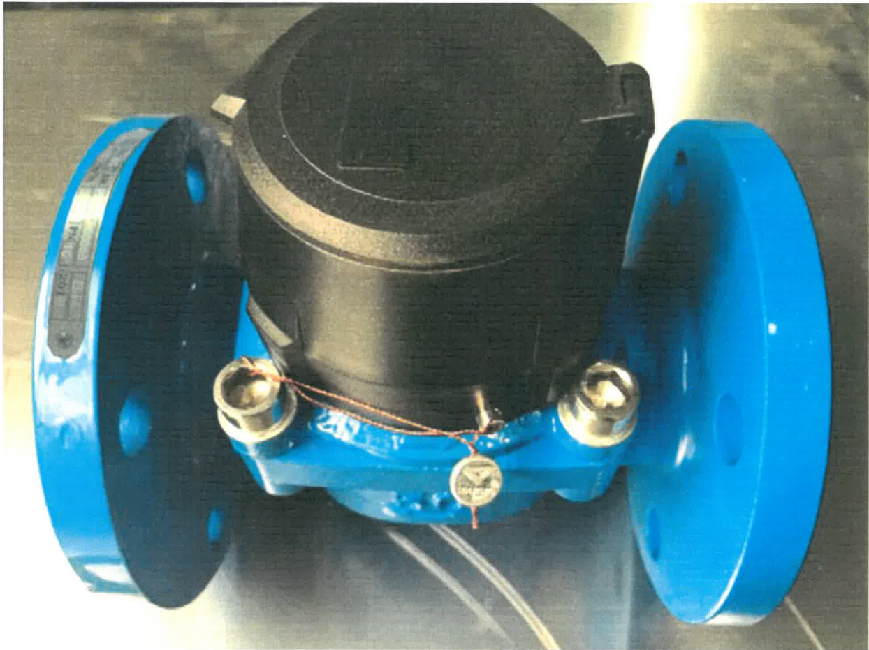
Figure 1: The water meter type CML – view and sealing:
